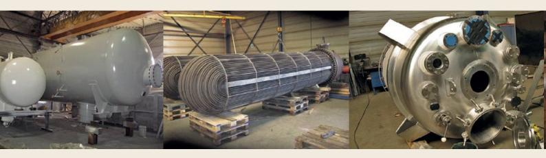
The equipment made using these more corrosion-resistant materials is produced either entirely from these materials, or using a coating technique whereby an expensive corrosion-resistant material is applied to relatively inexpensive base material, such as steel.
